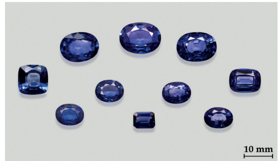
Fig. 1 10 diffused synthetic sapphires weighing from 1.69 to 10.46 cts. were used in this study. Photo by P. Ounorn 本研究採用的10顆經擴散處理的合成藍寶石，重量從1.69到10.46克拉。
